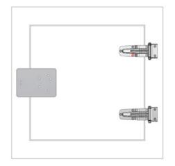
To adjust the anchoring piece, we need first to screw the two parts at their lowest position. If necessary, the next step is to elevate the upper vertical piece. This is done by moving the inferior piece to the left as shown in the picture and until the door is correctly adjusted.
